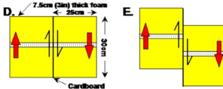
**Figure 1D and 1E. Strike-slip faulting using the foam model. Red arrows represent shearing. Half-arrows along faults show direction of relative motion along the fault plane.**
